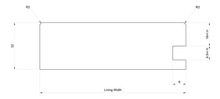
Description: Machining Profile - 32mm Timber Lining - NFR - Q2F To Pull
